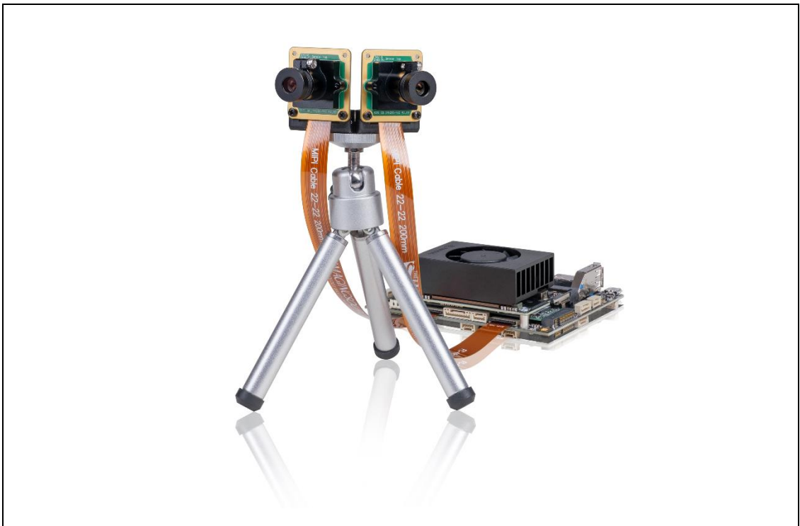
Figure 9: Connection of two MIPI CSI-2 cameras via a 22-pin 0,2 mm FFC cable incl. lens mount holder and M-12 lenses
