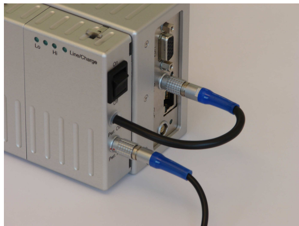
Schritt 6: Switch should be in positioned in „off“ state, connect camera and AccuPack
