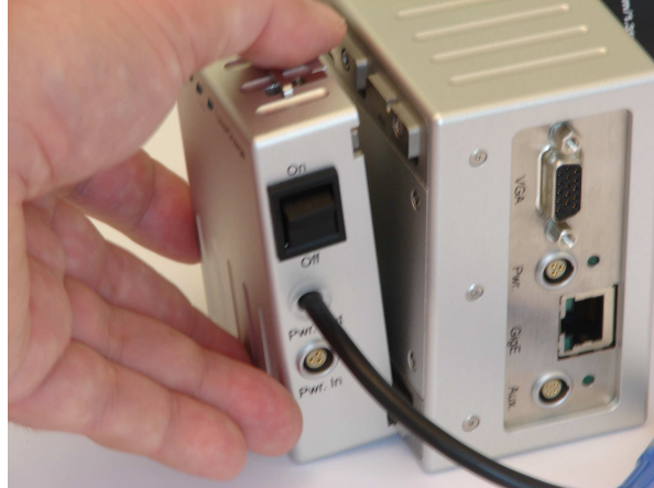
Step 1: Attach Charger to backside
