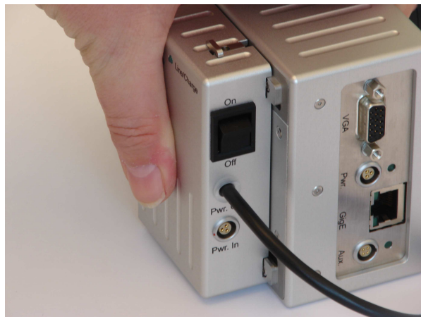
Step 2: Push Charger to backside
