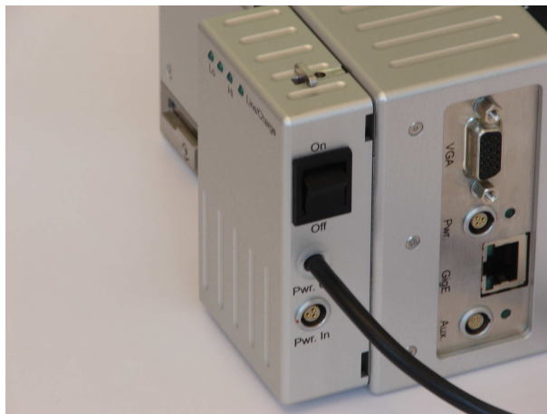
Step 3: Shift Charger into locking position
