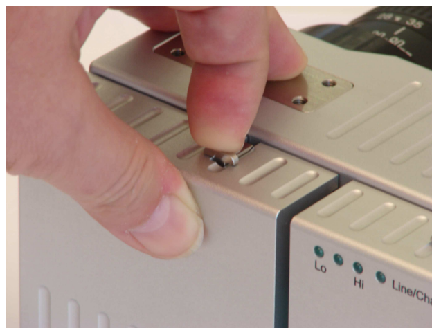
Step 9: ... and shift Accumulator to the left
