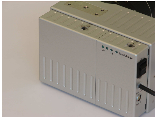
Step 5: Shift Accumulator to the right into locking position
