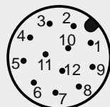
Power Supply / Digital-IOs (on camera side) (SACC-CI-M12MS-12CON-L180) wire colors of the connecting cable (ordered separately)
